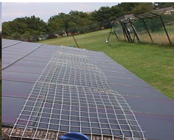
Figure 14 Shading 3a-Si with mesh
