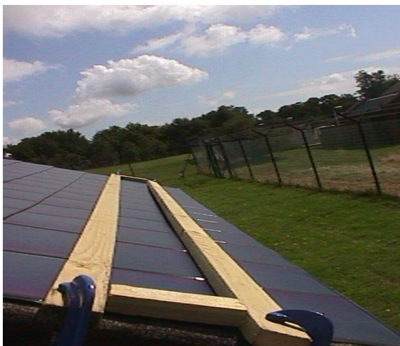
Figure 13 Shading 3a-Si with battens
