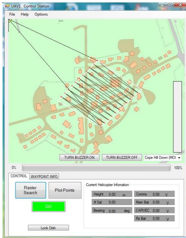
Figure 1. Mission control application, black lines indicate the flight path of the UAV over a village.
