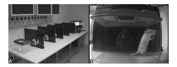
**Figure 2.** Use of the presented digital observation system for monitoring and recording rodent feeding behavior. **A**. Experimental setup and monitoring for 12 animals simultaneously, \* denotes circled example camera. **B**. Still frame of rat acquired using the presented digital observation system in normal light. **C and D**. A comparison of still frames taken by the analogue acquisition system (**C**) and the presented observation system (**D**) under red light conditions (~ 4lx).
