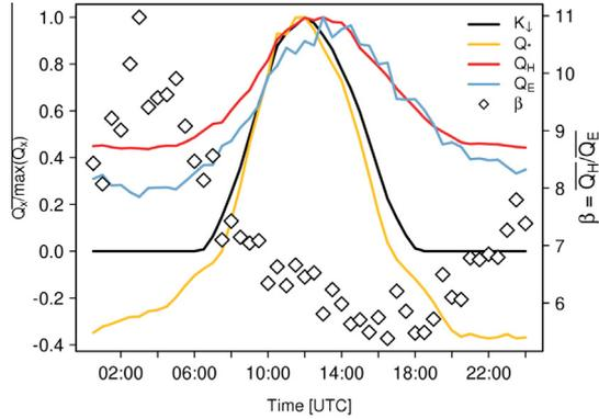
**Fig. 8.** Median diurnal pattern of energy fluxes  $Q_x$  at KSS, normalised by respective maximum  $\max(Q_x)$ : net all-wave radiation  $Q^*$ , shortwave incoming radiation  $K_i$ , and turbulent fluxes of sensible heat  $Q_H$  and latent heat  $Q_E$ . Bowen ratio  $\beta$  (diamonds) calculated from the median diurnal patterns of sensible and latent heat flux (restricted to  $|Q_E| > 3 \text{ W m}^{-2}$ ).
