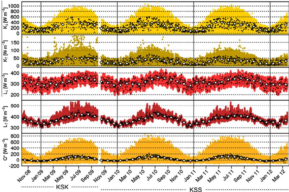
**Fig. 4.** Observations of the CNR1 net radiometer (after quality control) at KSK (10/2008–09/2009) and KSS (10/2009–03/2012): net all-wave radiation  $Q^*$  is the sum of incoming ( $\downarrow$ ) and outgoing ( $\uparrow$ ) long- ( $L$ ) and short-wave ( $K$ ) radiation, averages: 15 min (coloured dots), daily ( $K$ : daytime,  $L$  &  $Q^*$ : 24 h, black dots) and monthly (white diamonds). Data gap in October 2009 due to maintenance.
