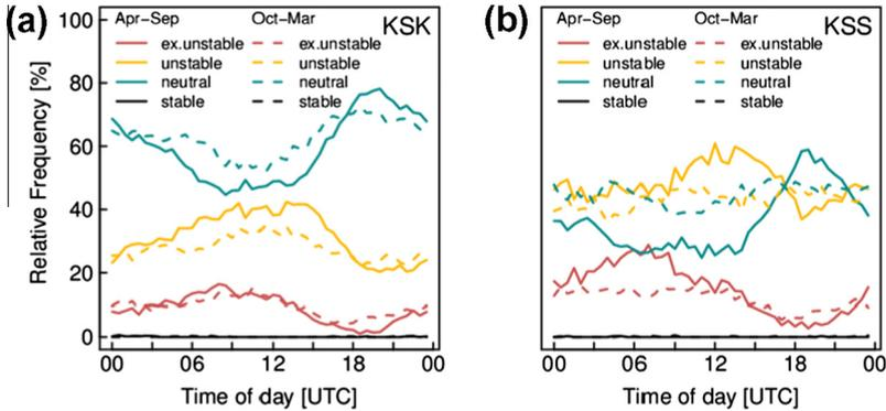
**Fig. 7.** Relative frequency of stability conditions by seasons or strength of sensible heat flux: spring/summer (Apr–Sep, stronger) and autumn/ winter (Oct–Mar, weaker) for (a) KSK and (b) KSS. See text for stability definitions.
