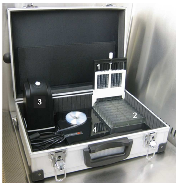
Figure 1. Main components of "Lab-in-a-briefcase" for PSA screening.
