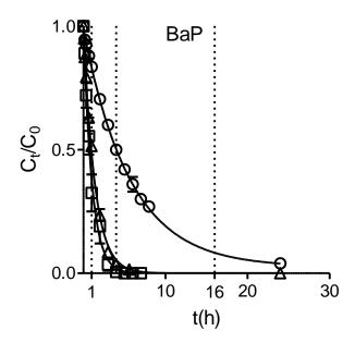
**Figure 3.** Elimination kinetics of PAHs from spiked simulated fluids into silicone rod. stomach ( $\Delta$ )small intestine ( $\Box$ )fluid and circle colon ( $\circ$ ). Data show mean PAH fraction of initial spike left in simulated fluid after time (t) of shaking at 37oC ± SEM (n= 2). Dashed lines indicate the incubation times in stomach (t=1), small intestine (t=4) and colon (t= 16) compartment of the extraction protocol.<sup>15</sup>
