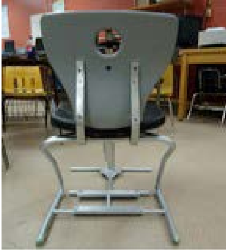
Figure 17. Fabricated seat and back support mounts.
