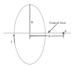
Figure 5-11: Graphical representation of the variables used Biot-Savart's Law
