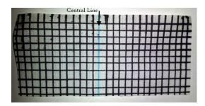
Figure 5-24: Rice paper gird used in surface flux density experiment
