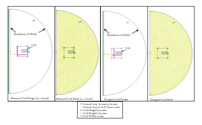
Figure 5-12: FEMM Models used to analyse the created coil
