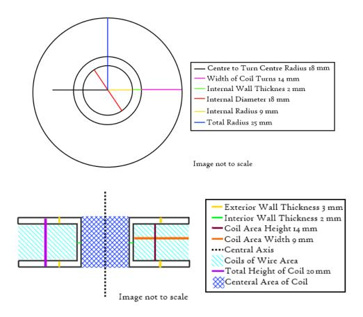
Figure 5-6: Electromagnet 'Stimulation' Coil Measurements. (Top) - Top down view, (Bottom) - Side on Cross Sectional View
