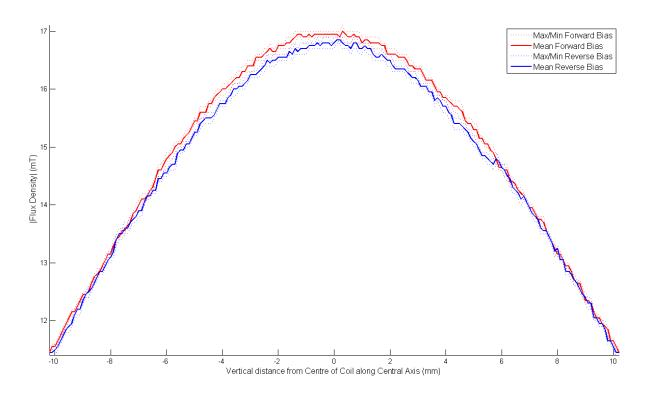
Figure 5-20: The magnitude of B field measurements recorded in the electromagnetic coil's centre along the central axis
