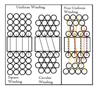
Figure 5-9: Uniform and non-uniform coil winding
