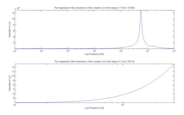
Figure 5-10: Impedance of created coil measured using a Bode 100
