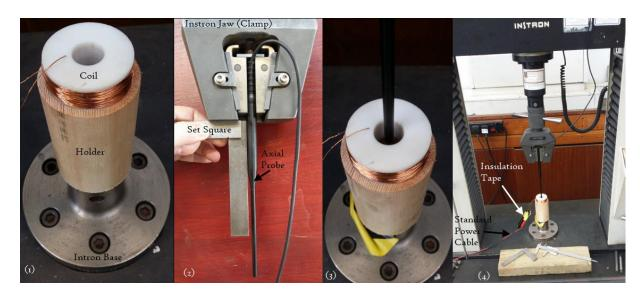
Figure 5-17: Experimental Setup Photographs. (1) - Coil in holder inside of Instron Base. (2) - Axial Probe in Instron Jaw (Clamp), alignment set with set square. (3) Probe Position in Coil. (4)
