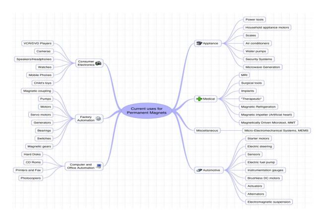
Figure 5-1: Uses of Magnets in Modern Technology [195, 196, 197, 198, 199, 200, 201, 202, 203]
