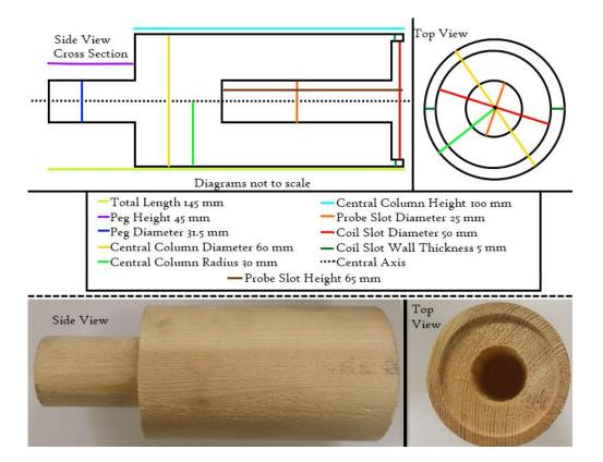
Figure 5-16: Wooden Holder used experimental approach of examining flux density of electromagnetic coil. (Top) – Schematic representation. (Bottom) – Photograph of holder.
