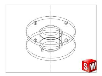
Figure 5-7: Wire frame view of the coil holder, developed in Solidworks
