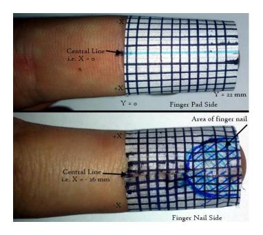
Figure 5-25: The author's fingertips with rice paper grid attached. X and Y values represent the measurement direction.
