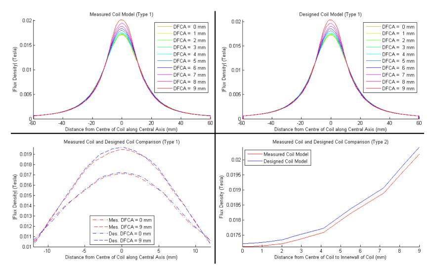
Figure 5-15: FEMM vector analysis. (DFCA – distance from central axis). Type 1 – Central axis and parallel vector measurements. Type 2 – perpendicular vector measurements from centre of coil to inner wall of coil.
