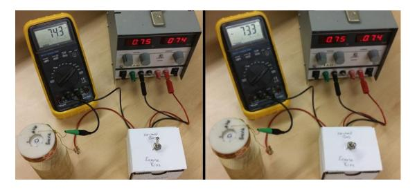
Figure 5-31: Flipping Experiment Electrical Experimental Setup. Left – Current in forward bias.
