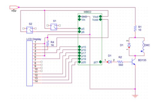
Figure 7-4: Circuit Diagram of Reaction Timer
