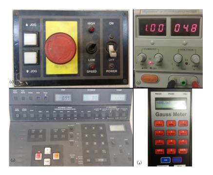
Figure 5-18: Instron Controls (1 & 2), Digimess Power Supply (3), Gauss Meter (4)
