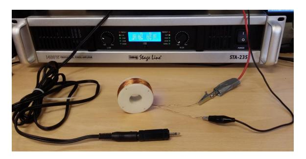
Figure 6-1: Power Amplifier, Audio Input Cable, Electromagnetic Coil and Power Leads for the Coil
