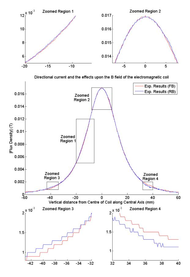
Figure 5-19: Magnitude of B field recordings observed along the central axis of the created electromagnetic coil. Exp. – Experimental, FB – Forward Bias, RB – Reverse Bias.
