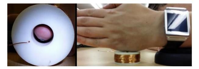
Figure 7-2: Fingertip location in coil (left) and Palmside hand location above the coil (right)
