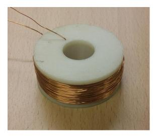
Figure 5-8: Electromagnetic 'Stimulation' Coil
