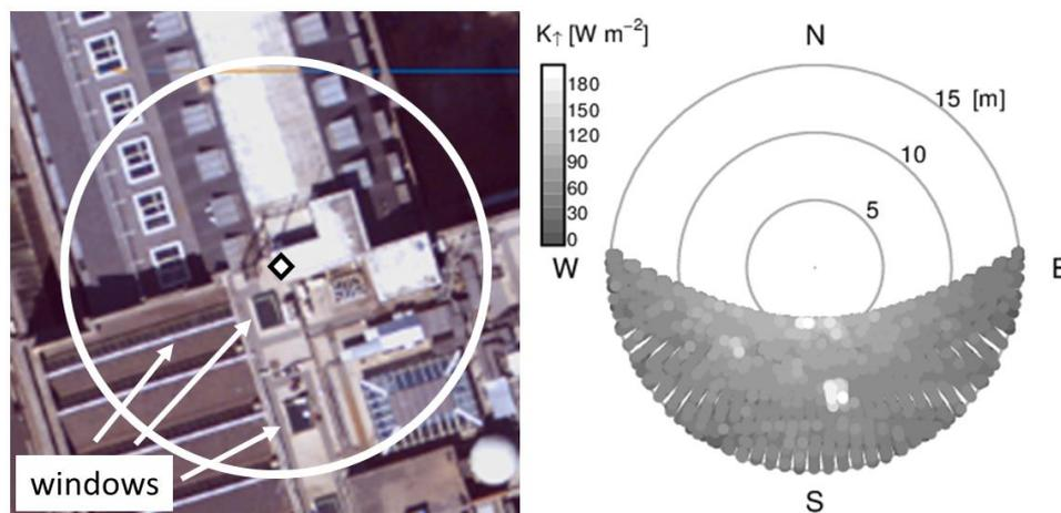
Figure 5: Effect of surface materials on reflected short wave radiation (a) circle shows 80% field of view (15.2 m radius) for the radiation sensor; (b) median reflected short-wave radiation observed (2012), by solar azimuth angle and distance of maximum, specular reflection  $R_s$ . Full details of analysis and definition of  $R_s$  in Kotthaus and Grimmond (2014b). Aerial photo (NERC ARSF 2008)
