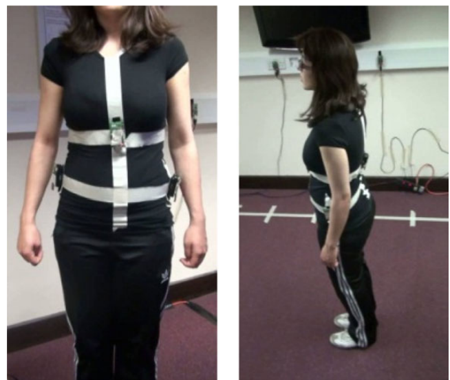
Figure 4. The test subject wearing the wireless modules.
