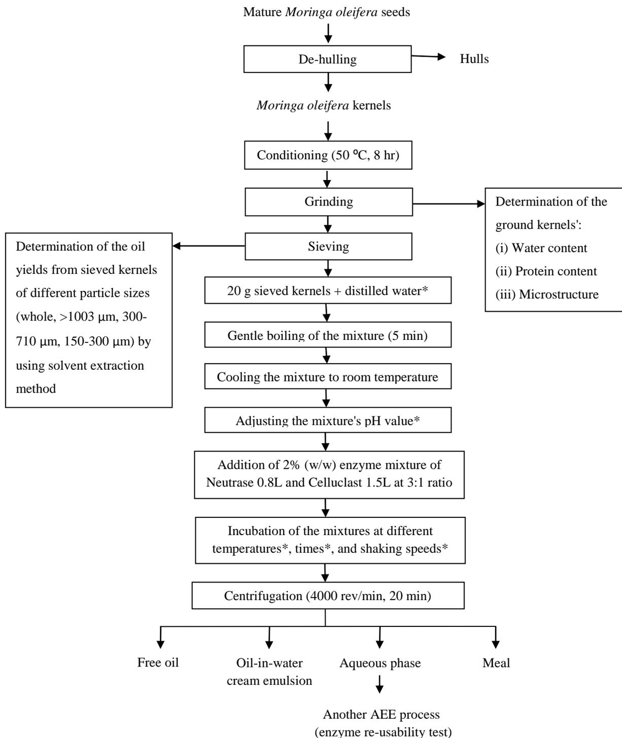
**Figure 3.1** Processes involved in the preparation of *Moringa oleifera* kernels, and extraction of *Moringa oleifera* oil via aqueous enzymatic (AEE) and solvent extraction methods. The (\*) represents the AEE parameters tested.
