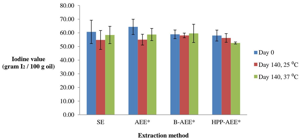
**Figure 5.7** Iodine value of *Moringa oleifera* oil from different extraction methods before (day 0) and after storage (day 140) at different temperatures. There was no significant difference ( $P > 0.05$ ) between all values. SE, solvent extraction; AEE\*, aqueous enzymatic extraction; B-AEE\*, aqueous enzymatic extraction with boiling pre-treatment; HPP-AEE\*, aqueous enzymatic extraction with high pressure processing pre-treatment.
