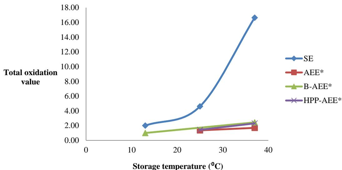
**Figure 5.4** Total oxidation (TOTOX) value of *Moringa oleifera* oil from different extraction methods after 120 days of storage at different temperatures. SE, solvent extraction; AEE\*, aqueous enzymatic extraction; B-AEE\*, aqueous enzymatic extraction with boiling pre-treatment; HPP-AEE\*, aqueous enzymatic extraction with high pressure processing pre-treatment.
