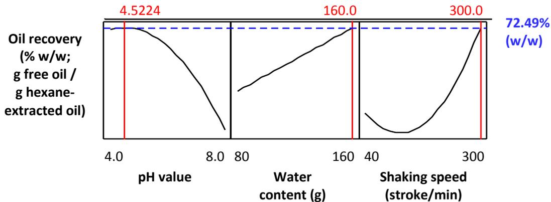
**Figure 3.5** The optimized aqueous enzymatic extraction (AEE) parameters (in red) which is predicted to yield in approximately 72.49% (w/w) *Moringa oleifera* oil recovery (in blue; g free oil / g hexane-extracted oil), and the effect of each parameter of pH value, water content, and shaking speed (in range) on the oil recovery; as generated by MINITAB<sup>TM</sup> Statistical Software: MINITAB Release 14.12.0, New York, USA, with modification.
