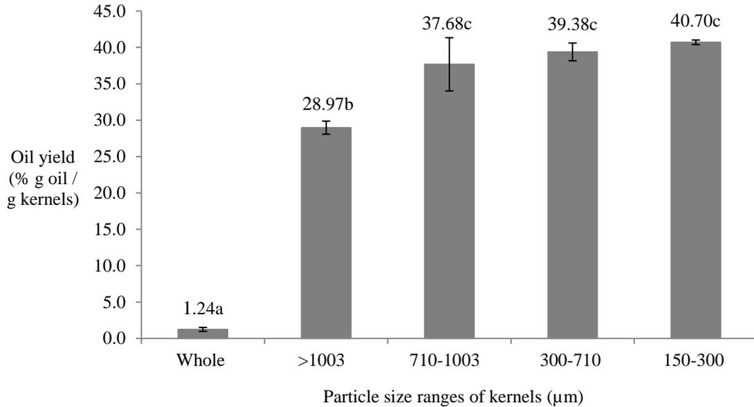
**Figure 3.2** *Moringa oleifera* oil yield from ground kernels of different particle sizes as determined by solvent extraction method using hexane. Mean values followed by different letters are significantly different ( $P < 0.05$ ).
