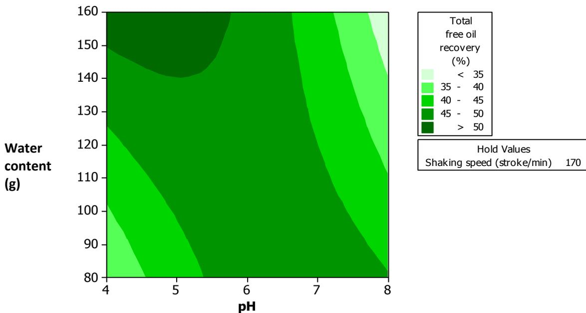
**Figure 3.6** Contour plot of the interaction effect between the pH value and water content (g) of a mixture undergoing an AEE process at 170 stroke/min incubation shaking speed on the free *Moringa oleifera* oil recovery (% g oil / g hexane-extracted oil) as generated by MINITAB™ Statistical Software: MINITAB Release 14.12.0, New York, USA with modification.
