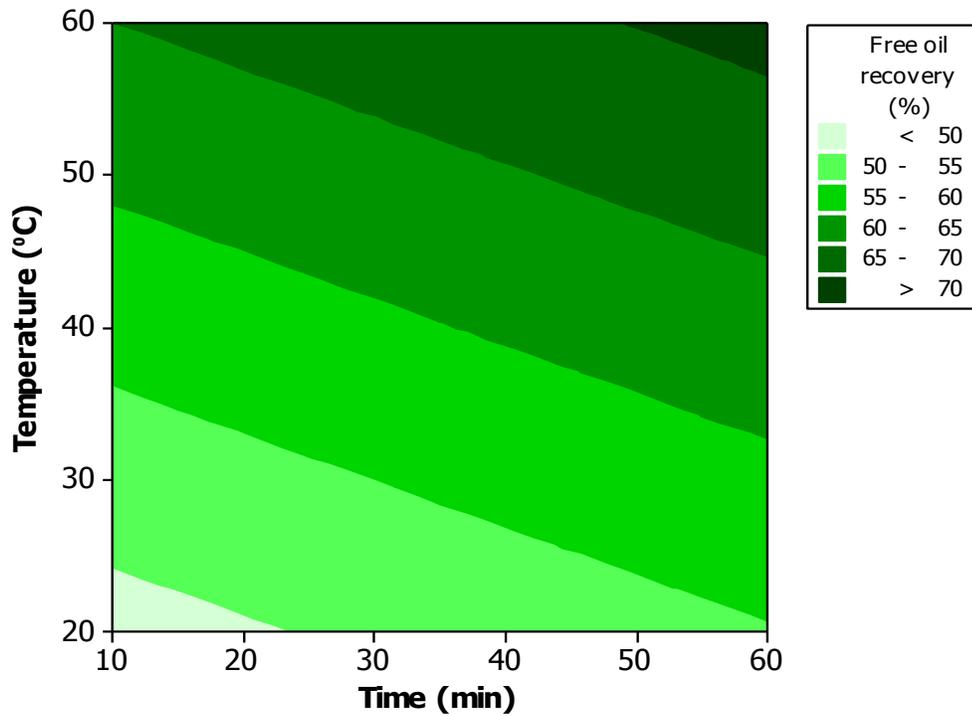
**Figure 4.3** The linear relationship between the high pressure processing (HPP) temperature and time as a pre-treatment on ground-sieved *Moringa oleifera* kernels prior to aqueous enzymatic extraction on the oil recoveries (% g oil / g hexane-extracted oil), generated by Minitab® 14.12.0 Statistical Software: MINITAB Release 14.12.0, New York, USA.
