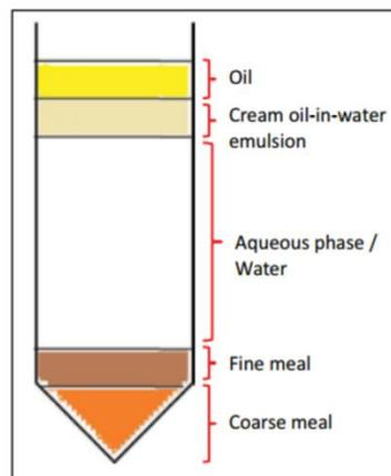
**FIG. 1.** Separation of different phases upon centrifugation after an aqueous enzymatic extraction method
