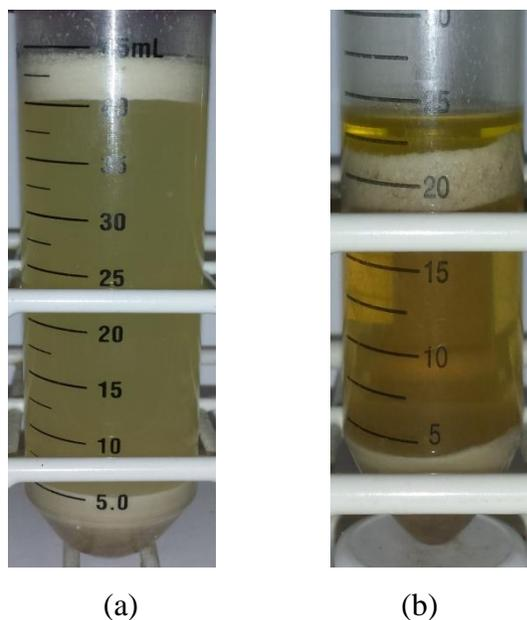
**Figure 3.9** The visual outcome after an aqueous enzymatic extraction (AEE) which was carried out by re-using the aqueous phase from (a) the optimized AEE and (b) Run 39. The parameters used for the re-usability tests were similar with that of the initial AEE process.
