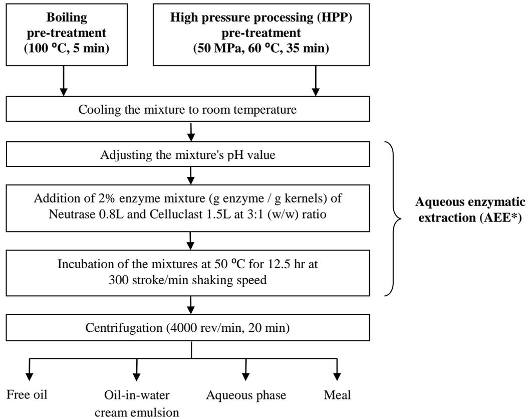
**Figure 4.4** The new experimental procedure to determine the effect of boiling and high pressure processing pre-treatments prior to the aqueous enzymatic extraction (AEE\*) method. The AEE\* with boiling pre-treatment is termed as B-AEE\*, while the AEE\* with high pressure processing pre-treatment is termed as HPP-AEE\*.
