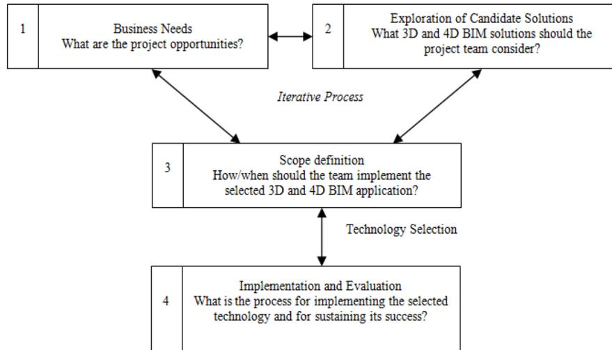
Fig. 3: Proposed 4D model to optimize IPD process
