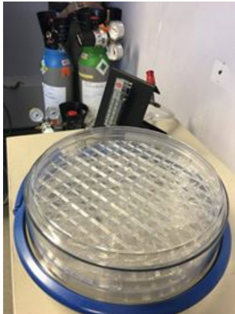
Figure 2-5 The Modular Incubator Chamber MIC-101 connected to gas cylinders with a two-stage regulator.
