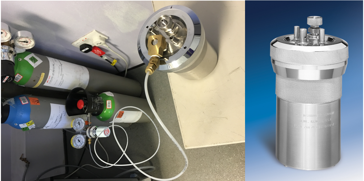
Figure 2-3 The oxygen combustion vessel and the connection unit that connected to the gas cylinder.
