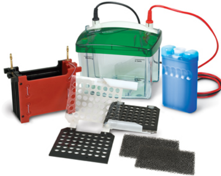
Figure 2-10 The Mini Trans-Blot cell Apparatus including the transfer tank, transfer blot, cooling pack and transfer cassette.
