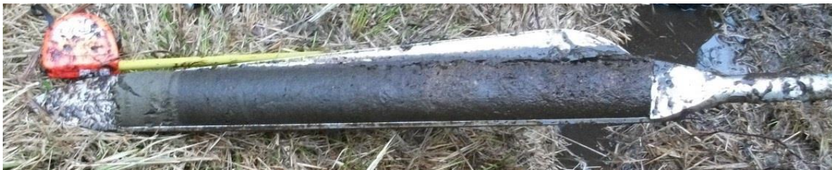
Figure 4.13. A sampled core taken using the 500mm x 50mm Russian Corer.
