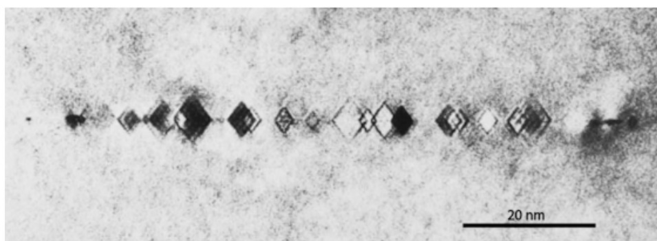
Figure 9. Voidite sheet in type Ia diamond. Reproduced with permission from [64]. Royal Society, 1987.
