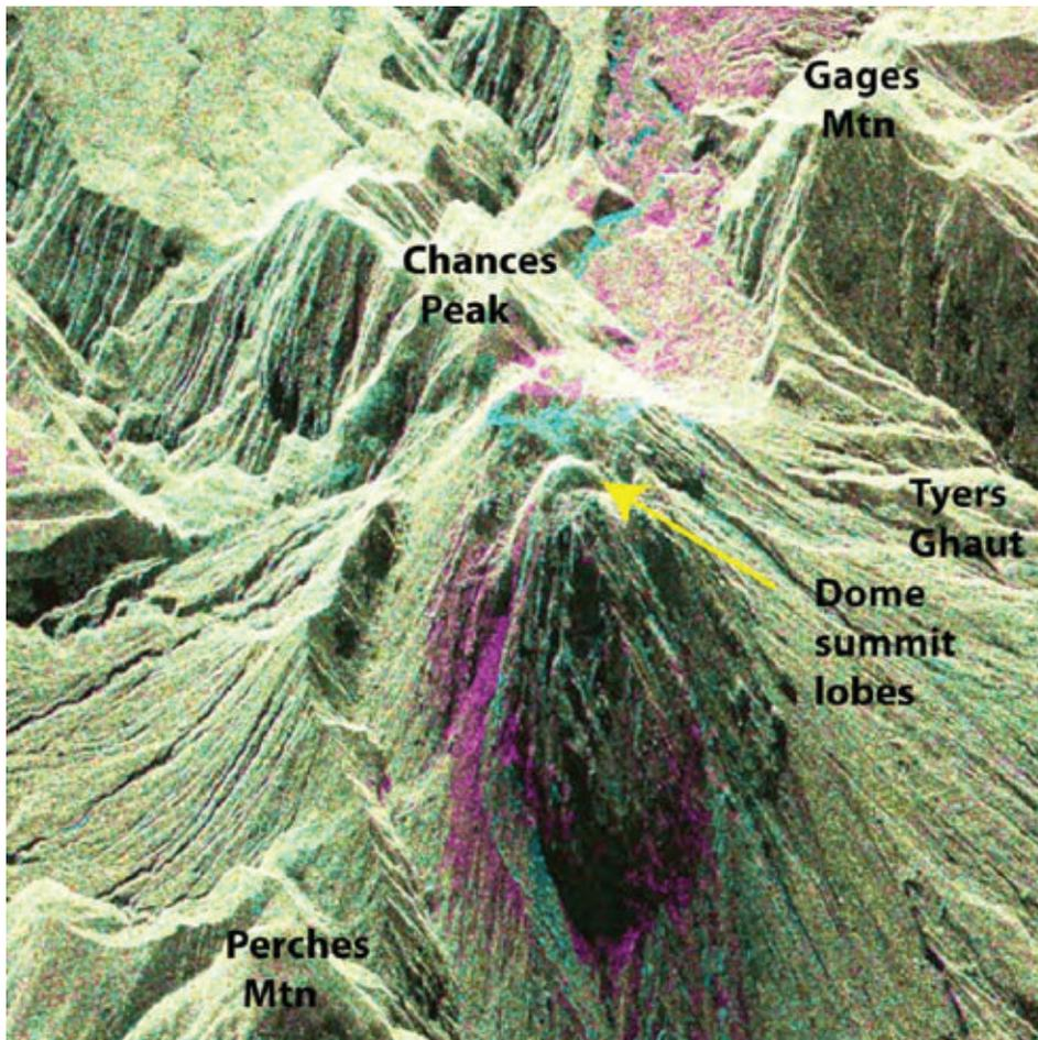
**Figure 3** Change difference TerraSAR-X image of Soufrière Hills volcano using full resolution (approximately 2m) slant range data with no topographic correction. This is the equivalent data of Figure 1 with the orientation rotated through 90 degrees (west is up). The colour interpretation is as for figures 1 and 2. (Image © DLR 2008, annotation G. Wadge).
