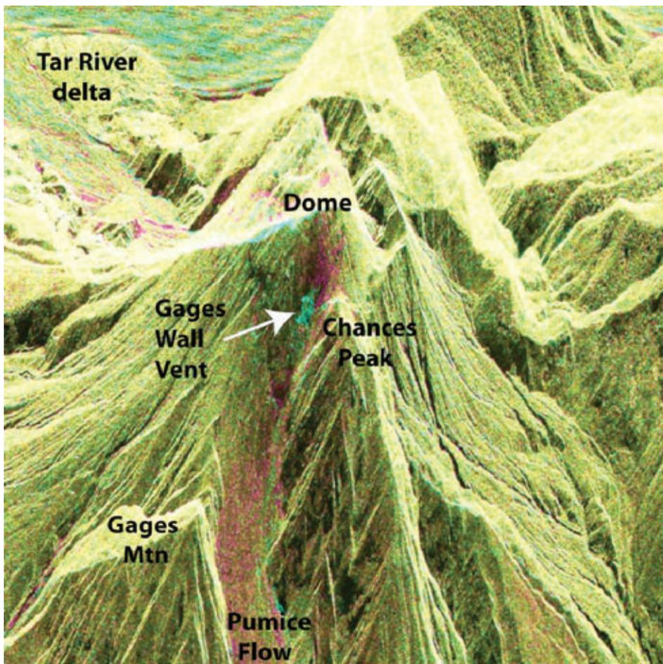
**Figure 4** Change difference TerraSAR-X image of Soufrière Hills volcano using full resolution (approximately 2m) slant range data with no topographic correction. This is the equivalent data of Figure 2 with the orientation rotated through 90 degrees (east is up). The colour interpretation is as for Figures 1 and 2. The cyan area is the Gages Wall vent expanded during the 28/9 July explosion. (Image © DLR 2008, annotation G. Wadge).
