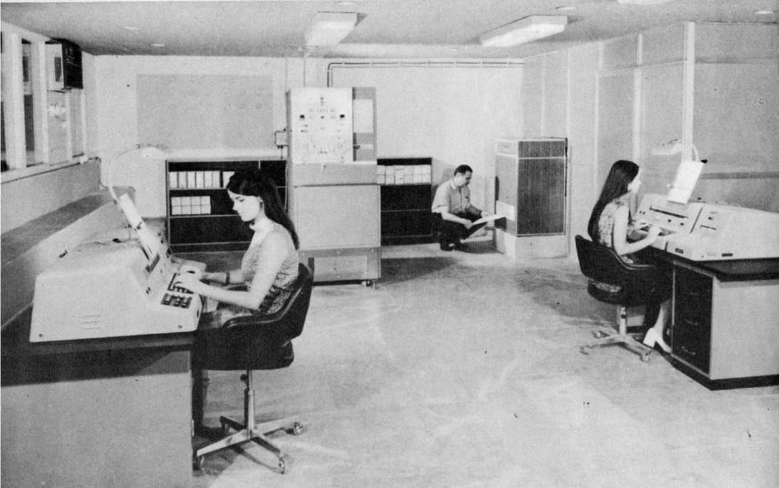
Figure 4.3. The installation of the Linofilm Super-Quick at APC shows the different units that comprised the phototypesetting system. On the right, the keyboard operator is T. Papanikolaou (née Tsimidopoulou), manager of the photocomposition department at APC, G. Varanakis is by the film unit at the back, and C. Natsis, editor of the *DA Review*, sits at the keyboard of the perforating machine on the left. CADA. 77% of original size.
