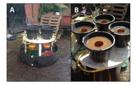
Image 2.3. Root washer apparatus. A) Side view of root washer showing collection filters and buckets on table surface, containing soil samples. B) Top view of root washer showing jet pumps filling buckets containing soil samples. Water containing wheat roots passes through hollow cylinder in bucket and into collection filters.
