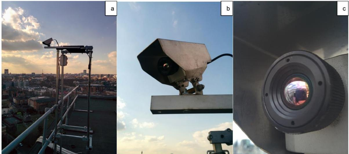
Figure E-1. Example setup of Optris PI-160 LWIR camera (years 2015-16) at the IMU site with (a) overall mounting of south facing camera (photo looking southwest) (b) close-up of the Optris PI-160 camera in original aluminium housing, and (c) front of the camera within the aluminium housing.
