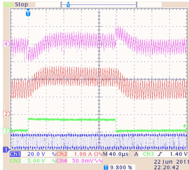
(a) Measured transient response of analog system.
