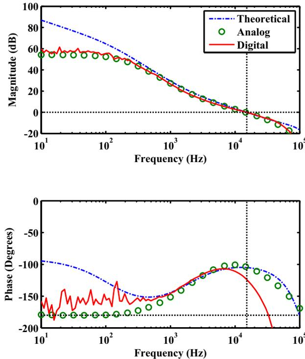
Fig. 11. Measured open loop frequency response at full load, 16W, using an OMICRON Lab Bode 100 vector network analyzer. Crossover frequency/phase margin: Analog 15kHz,  $76^\circ$ . Digital 15kHz,  $58^\circ$ .
