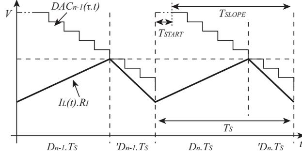
Fig. 4. Slope compensation using a digital staircase.
