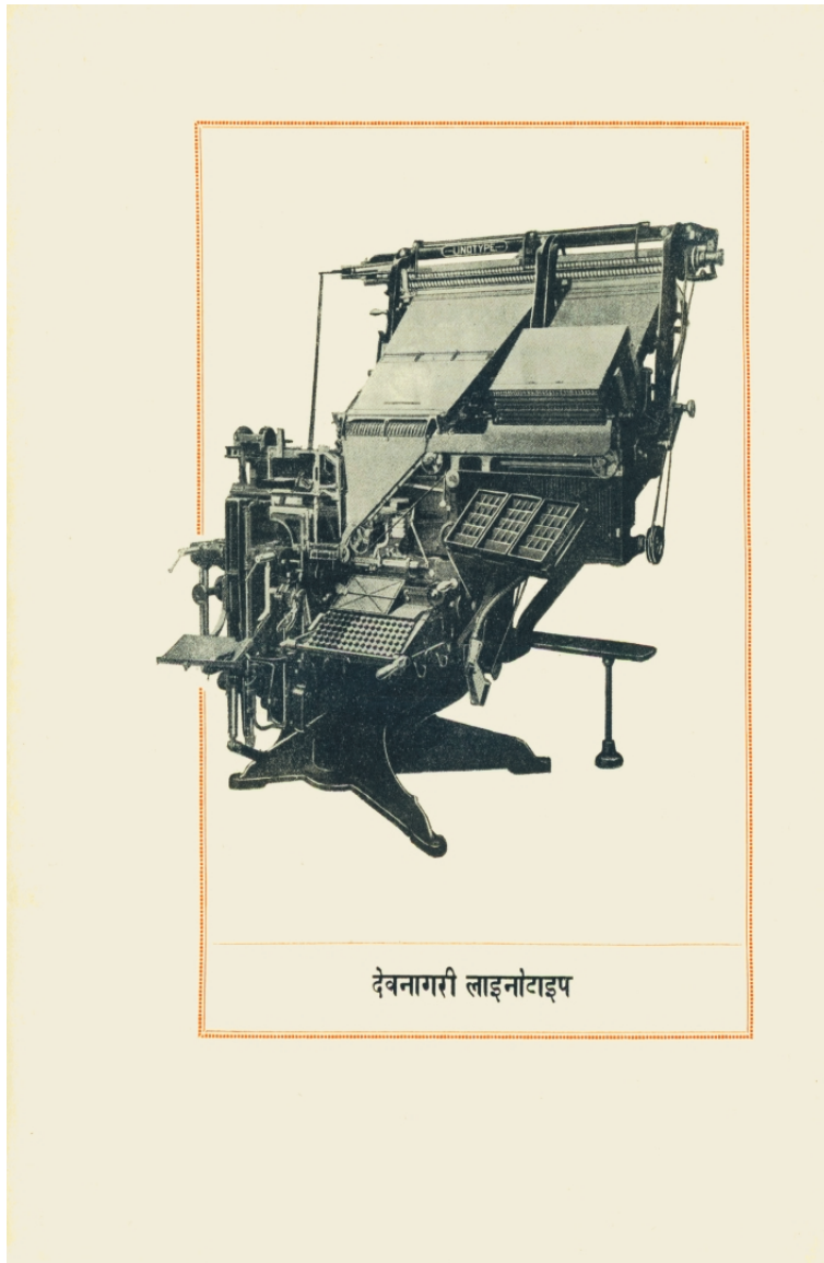
Fig. 4b. Page showing the Linotype machine for Devanagari from Announcing Devanagari Linotype (New York: Mergenthaler Linotype Company, 1933). Reduced from 265 × 193 mm.
