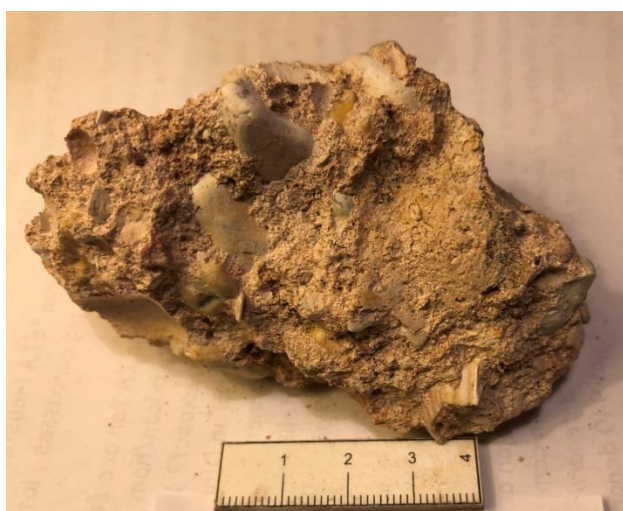
Fig. 1. Hand specimens of mortar Sample 1 (42) prior to sampling for thin section (scale cm).
