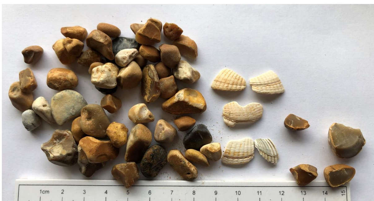
Fig 9 Gravel from modern Hythe beach with rounded flints and cockle fragments. At right fractured gravel shows patinated and iron-stained surfaces
