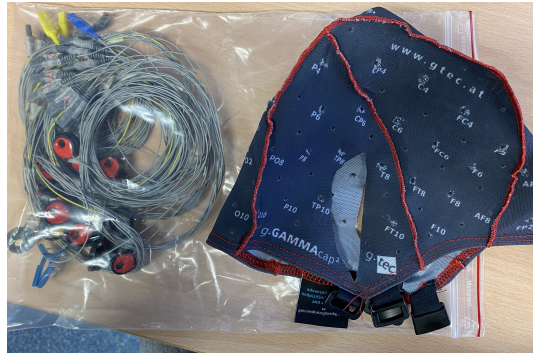
Figure 6.2: 32-electrode EEG cap (g.GAMMA cap, g.tec medical engineering GmbH Austria)
