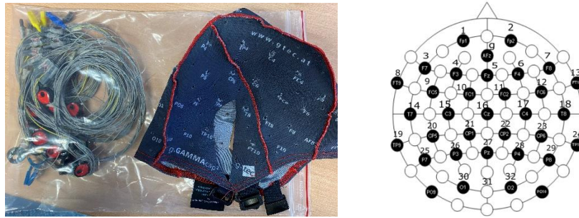
Figure 2. The EEG cap and the locations of the 32 EEG channels
