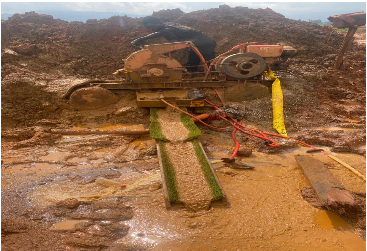
Plate 6: A full set up of a 'champhyne' (ASM machine for processing the gold ore)
