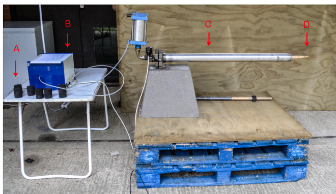
Fig. 4. Air cannon experimental setup. A: foam discs used to create a seal between the spear and the barrel. B: The air cannon controller. C: the barrel within which the replicas sit. D: the front point of a wooden spear replica.
