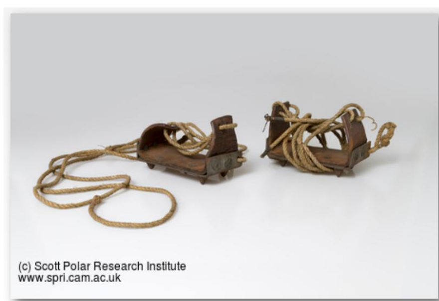
Figure 4.8. N: 103a-b - A pair of crampons made in England for the British National Antarctic Expedition 1901-04 (Discovery). The design was found to be unsuitable as it allowed snow to get between the footwear and the crampon © SPRI.
