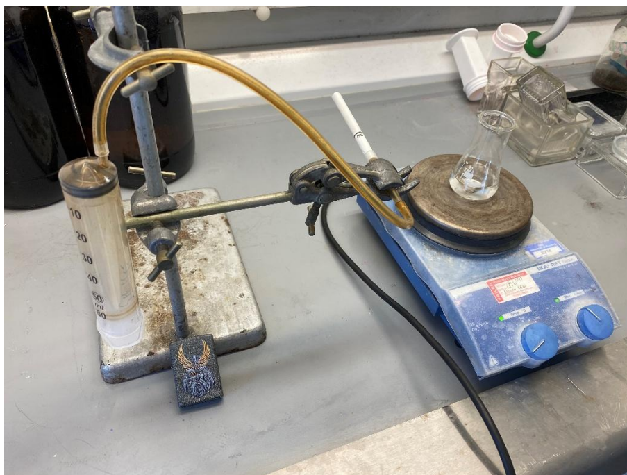
Figure 2.1. Setup used to extract cigarette smoke media.
