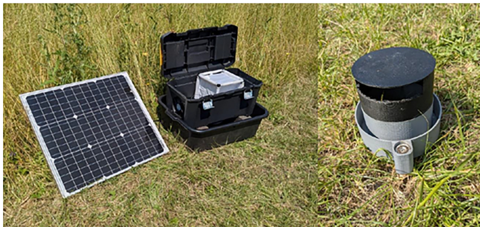
FIGURE 1 Box-Gravid trap. Left: viewed with lid open, showing the BugDorm container housing trapped mosquitoes and the FTA™ card; outlet fan, photovoltaic panel and black water container are also shown. Right: 3D printed intake pipe, providing access for adult mosquitoes into the BugDorm and preventing mosquitoes falling back into the water.
