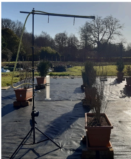
(C). Rainfall applicator and a tripod stand
