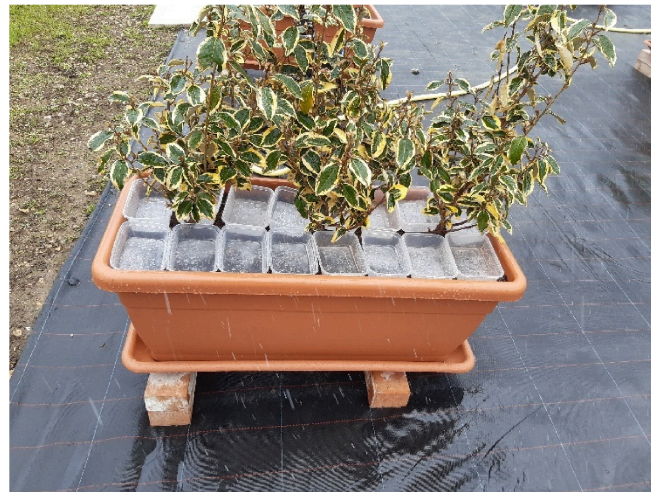
Figure 2. Position of containers collecting runoff from canopies during and after 5 min simulated rainfall application.
