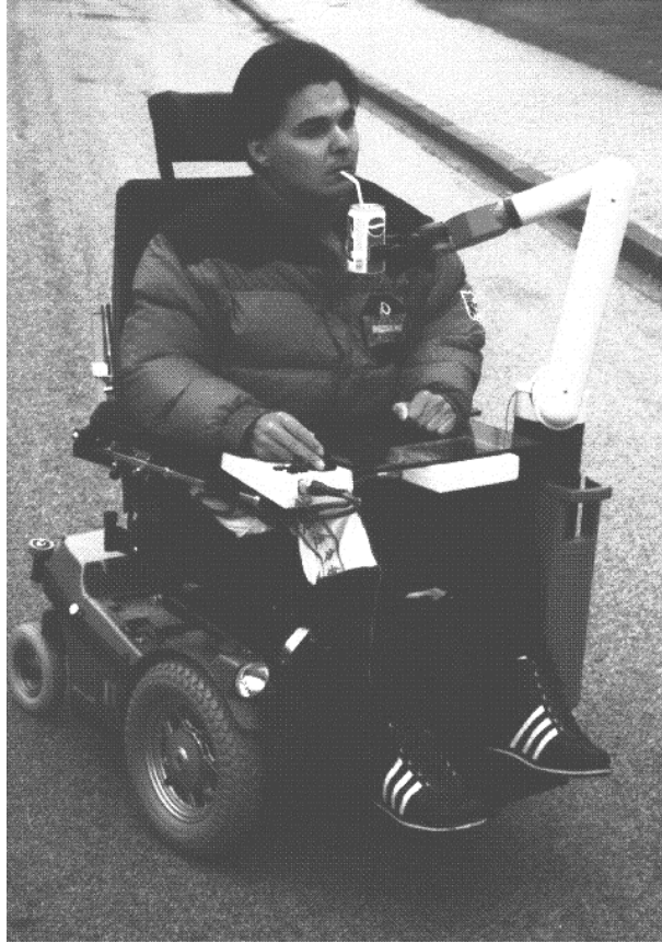
Figure 1. Manus manipulator mounted on a wheelchair.
