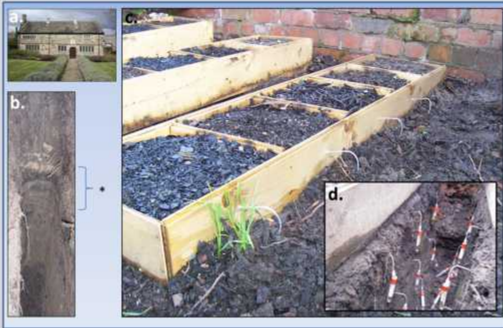
838 Figure 9. Urban soil study site showing a.) view of the garden where experimental trenches were 839 located, b.) excavated soil profile revealing now buried deposits of heavy metal rich soot at the 840 surface of the soil circa. industrial era (marked *), c.) surface amendment matrices and d.) pore 841 water samplers in place at 25, 50 and 75 cm depth.
