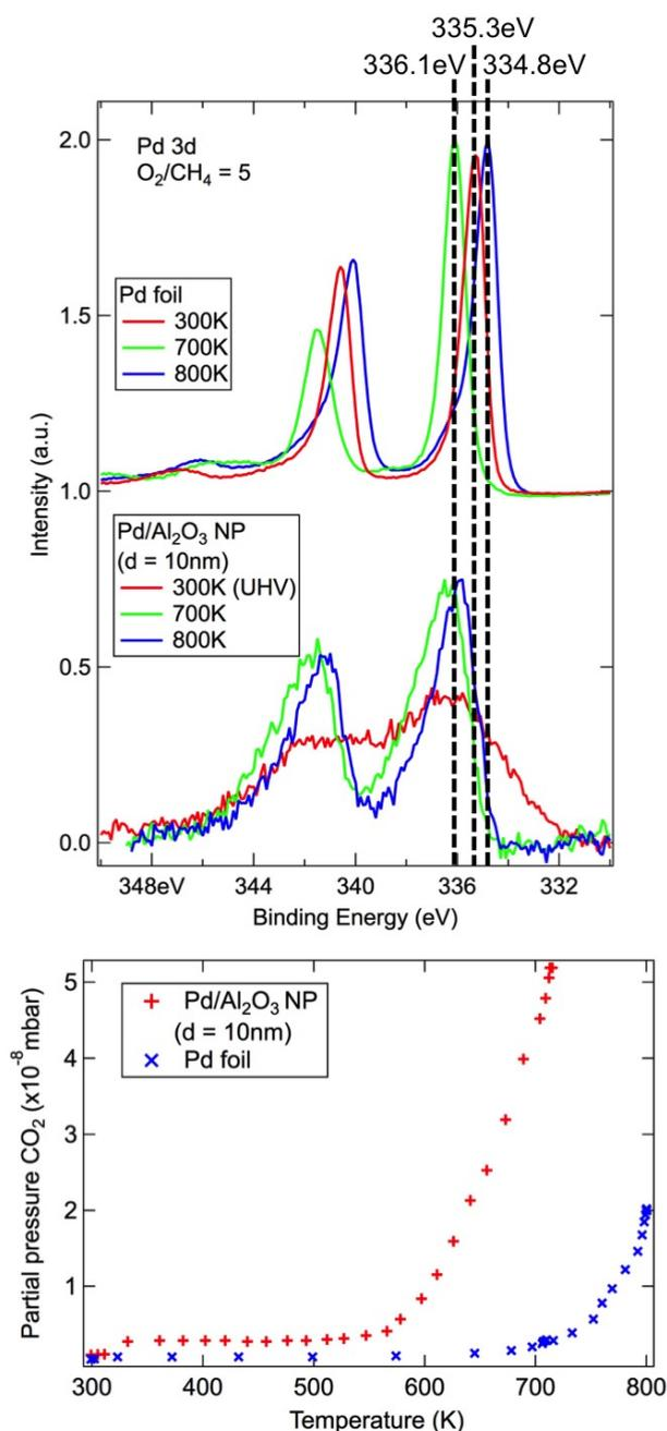
**Fig. 7** Comparison of polycrystalline Pd foil and Pd/Al<sub>2</sub>O<sub>3</sub> nanoparticles calcined to 600°C ( $d = 10$  nm): AP-XPS spectra and partial pressure of CO<sub>2</sub> produced under O<sub>2</sub>/CH<sub>4</sub> = 5 (total gas pressure = 0.33 mbar/240 mTorr) at 300 K, 700 K and 800 K.
