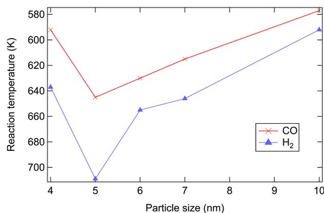
**Fig. 6** Temperature of CO and H<sub>2</sub> initial production vs. particle size.
