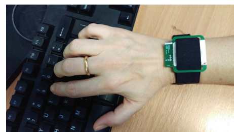
FIGURE 2: Prototype inertial measurements logger (as worn (×5) by participants).
