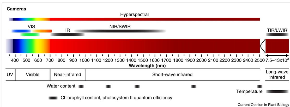
**Fig. 1.2 – Wavelengths of the visible spectrum (VIS), the infrared spectrum (IR), the near-infrared (NIR) and the long-wave infrared (LWIR). Source: Fahlgren *et al.* (2015).**
