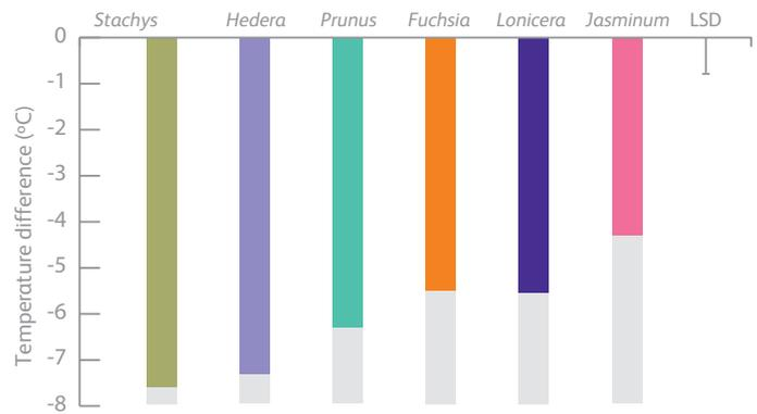
Figure 7.2: The extent to which different plant species can provide cooling to a building wall. The use of plant screens can reduce the amount of solar irradiance impacting on a building, thus reducing the requirement for artificial air conditioning. Comparison of a range of wall shrubs/ climbers with *Stachys* as a comparison (Cameron et al. 2014).
