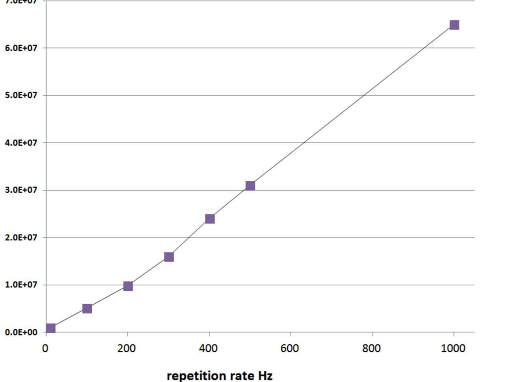
Figure 5: bradykinin  $[M+2H]^{2+}$  signal (arbitrary units) as a function of laser pulse repetition rate up to 1kHz (at 14  $\mu\text{J}$  per shot).
