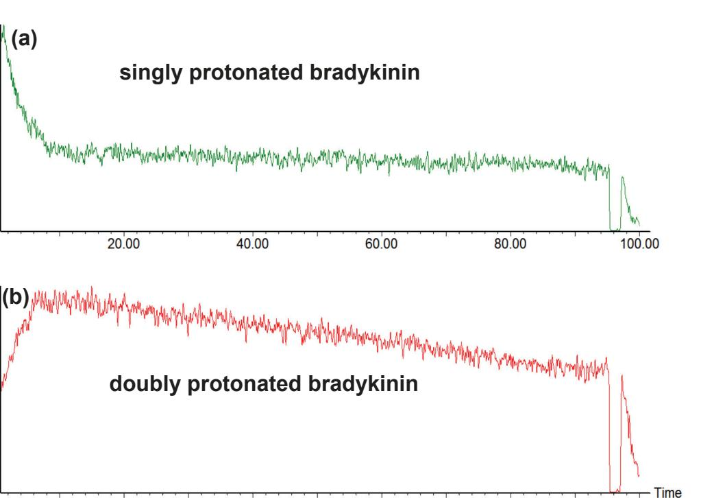
Figure 3: A single micro-litre of sample/matrix solution produces (a)  $[M+H]^{+}$  and (b)  $[M+2H]^{2+}$  signals for more than 90 minutes when irradiated at 10Hz laser pulse repetition rate.
