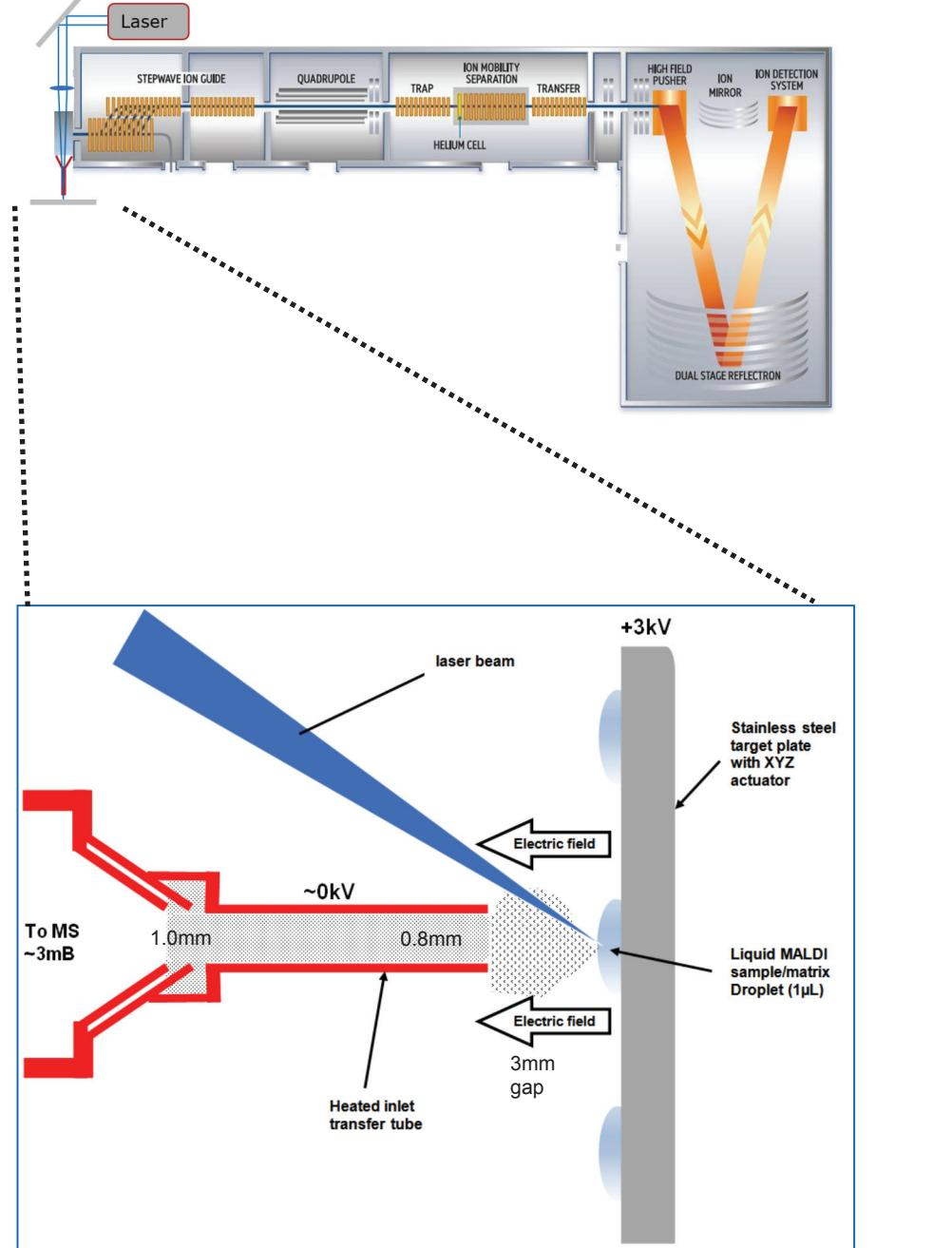
Figure 1. Modified Synapt G2-Si system with the ESI source replaced by an experimental AP-MALDI source assembly including XY sample plate and heated inlet capillary
