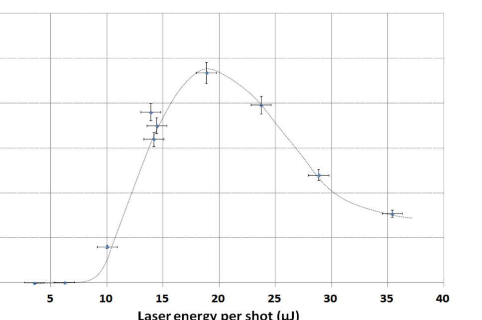
Figure 2. Signal intensity (arbitrary units) per laser shot for bradykinin  $[M+2H]^{2+}$  as a function of laser energy at 10Hz laser pulse repetition rate. The ionisation threshold was at an energy of 6  $\mu\text{J}$  and the maximum signal was at 18  $\mu\text{J}$ .
