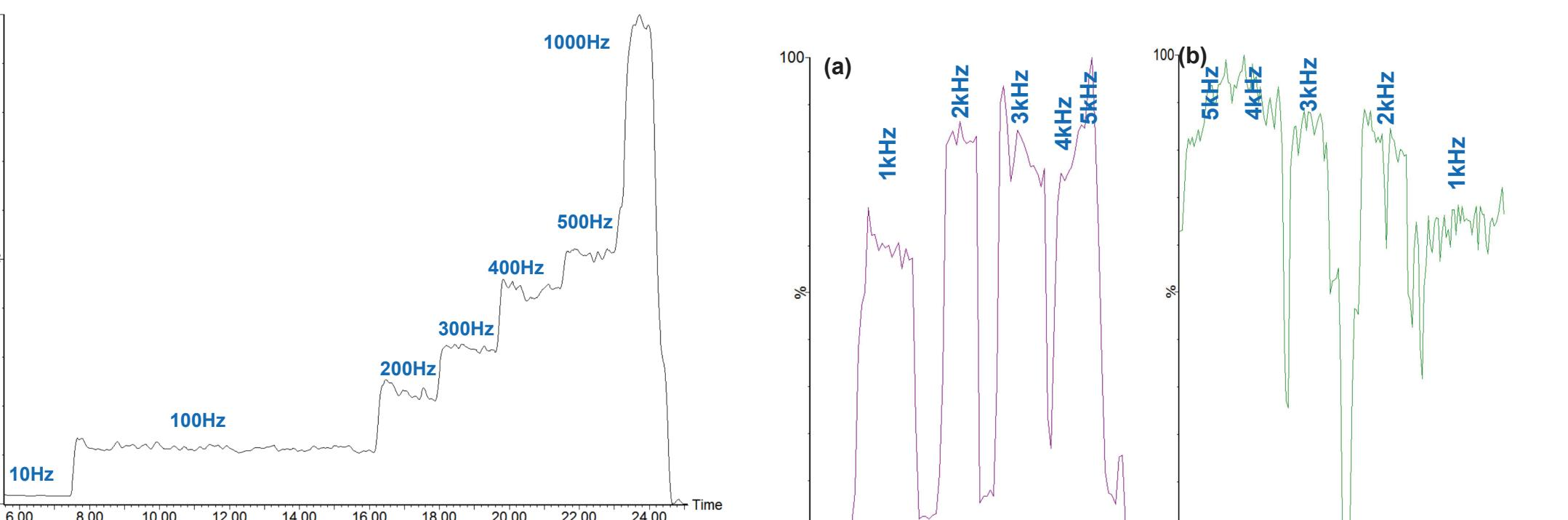
Figure 6b: Chromatograms of doubly protonated bradykinin at a) increasing repetition rates from 1kHz to 5kHz and b) decreasing repetition rates from 5kHz to 1kHz. Note the excessive signal fluctuation compared to Figure 4.
