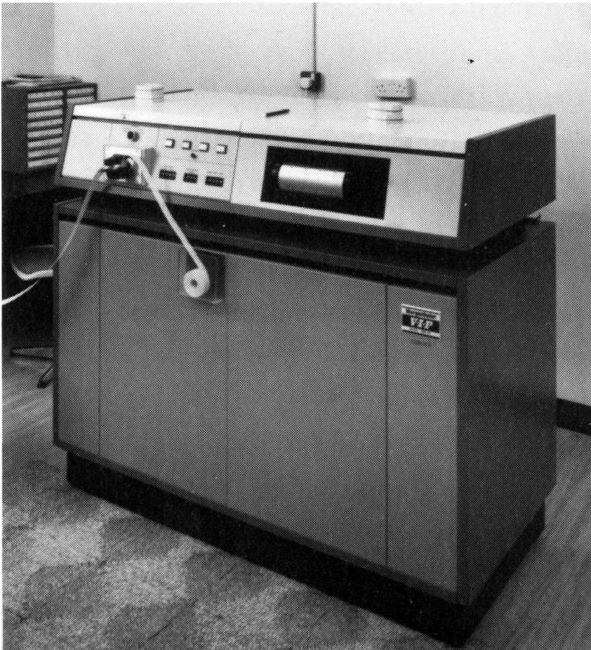
Figure 6.1. The Linofilm Variable Input Phototypesetter (V-I-P). The device was popular with medium- to large-size printing businesses and newspapers, and helped establish Linotype as a major manufacturer of phototypesetting equipment. It was also ideal for setting Greek as it enabled the easy centring of accents. From Wallis, *Typomania*, 52. 250% of original size.
