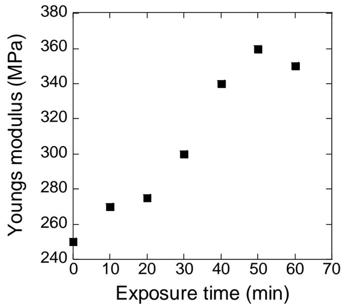
**Fig. 8.** The variation of Young's modulus with exposure to UV light of intensity  $10 \text{ mWcm}^{-2}$  and wavelength 365 nm.
