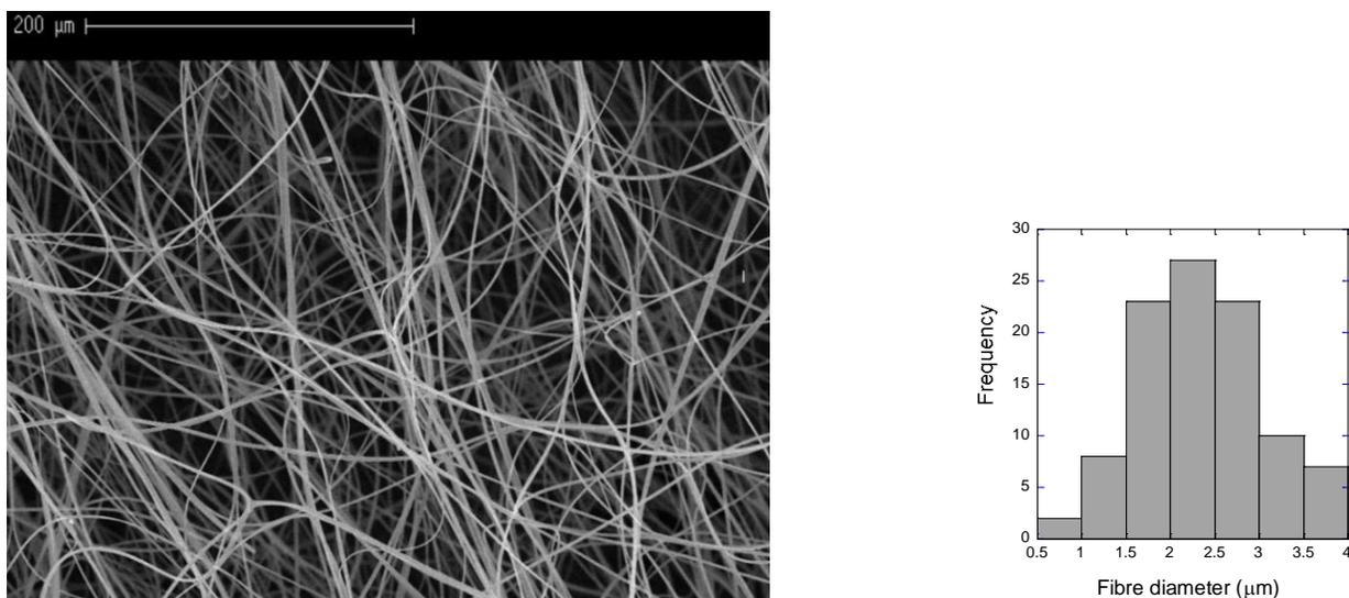
**Fig. 2.** Topology and distribution of nonirradiated PVCN fibres (Cambridge S360 SEM). The needle-collector separation was 10 cm and a voltage of 17 kV was maintained between them. The average fibre diameter is  $2.36 \pm 0.70 \mu\text{m}$  and this represents the average of 100 measurements randomly selected from across the SEM image.
