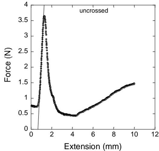
**Fig. 7.** The stretching force versus extension for uncrossed PVCN fibres was measured with a Deben tensiometer which is fitted with a 200 N tensile stage. The dimensions of the bundle were: 10 mm x 0.4 mm x 0.4 mm and the stretching rate was 0.5 mm min<sup>-1</sup>. The Young's modulus is calculated from the slope of the linear region shown.
