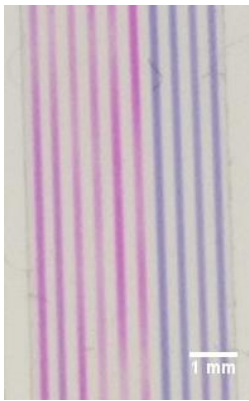
An image of the colour change in a microcapillary indicating bacterial growth
